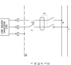
X1....X3 CLAMPS SWITCH (EVENT. CONTACTOR REGULATED BY THERMOSTAT) CURRENT GUARD
