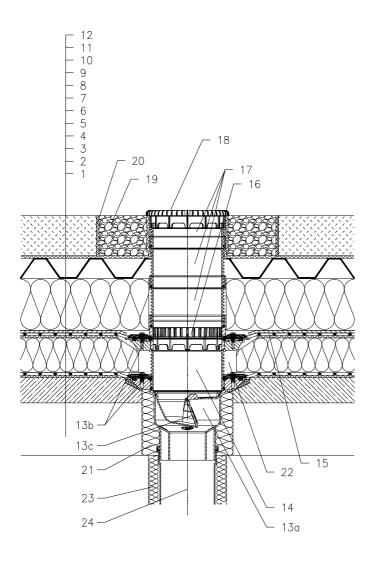
TO HEAT THE DRAIN, YOU MAY USE HEATING KIT HKL156 WITH REGULATING HEAT SOURCE 40W/M; 230 V; (APR. 12-14W HEATING TAPE). (THE HEATING TAPE INCL. THERMAL INSULATION MUST BE PULLED ON THE DRAIN BODY BEFORE INSTALLATION) RECOMMENDED BOREHOLE DIAMETER IS \$020mm,\(\frac{1}{2}\)220x220mm.
