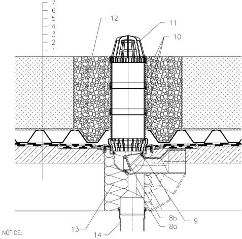
TO HEAT THE DRAIN, YOU MAY USE HEATING KIT HL82 WITH SELF-REGULATING HEAT SOURCE 18W/220V. (THE HEATING TAPE MUST BE WRAPPED AROUND THE DRAIN BODY BEFORE INSTALLATION).
