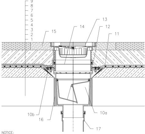
TO HEAT THE DRAIN, YOU MAY USE HEATING KIT HL609 WITH SELF-REGULATING HEAT SOURCE 36W/23OV. (THE HEATING TAPE MUST BE WRAPPED AROUND THE DRAIN BODY BEFORE INSTALLATION).
